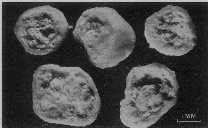
Figure 5. Granules of 14-14-14 leached-zone fertilizer cleaved to show hulls of potassium nitrate and ammonium chloride that developed during storage
